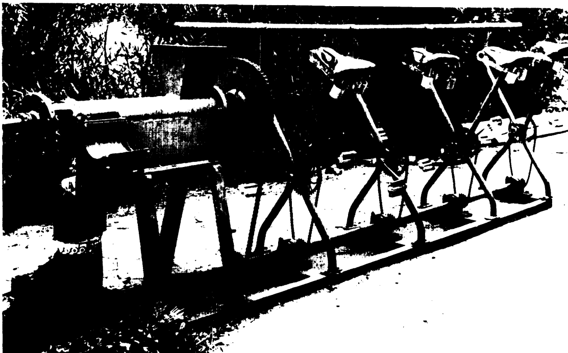
Figure 16.—Screw Press Operated by Human Power in India
