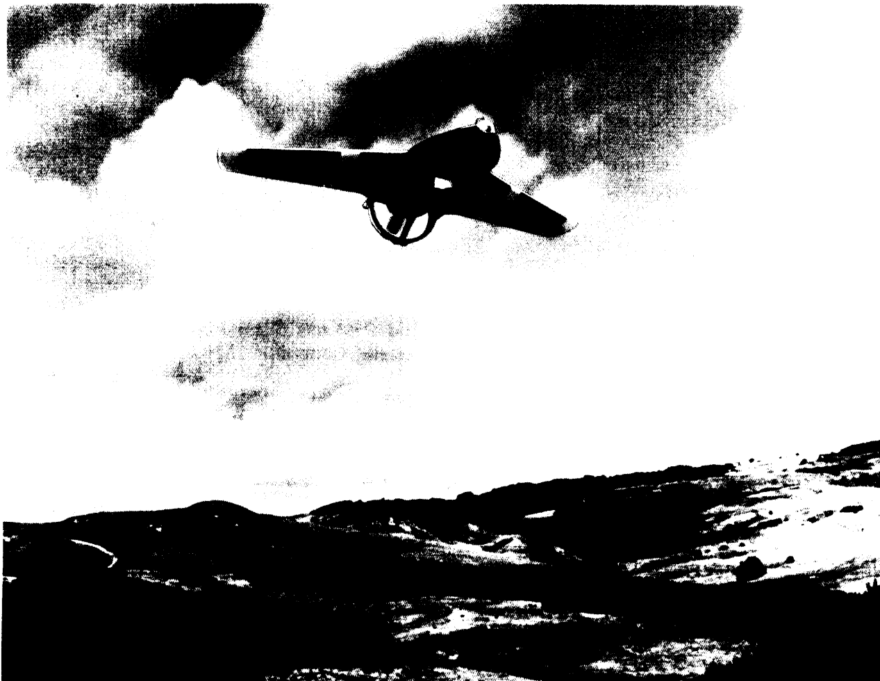
Figure 10-3.—The Aquila Remotely Piloted Vehicle
