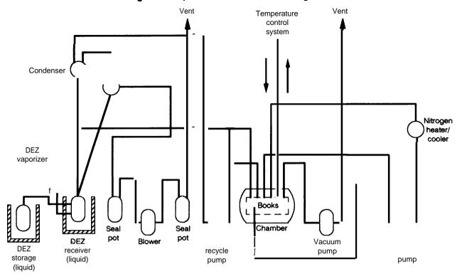
Figure 6.-Simpltfied DEZ Process Flow Diagram
