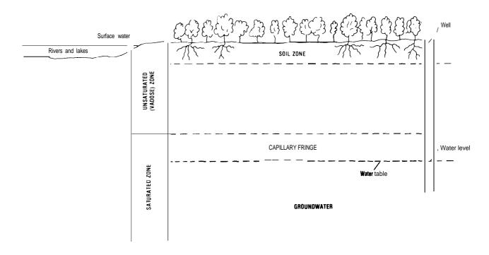
Figure 3-2—Zones of Subsurface Water
