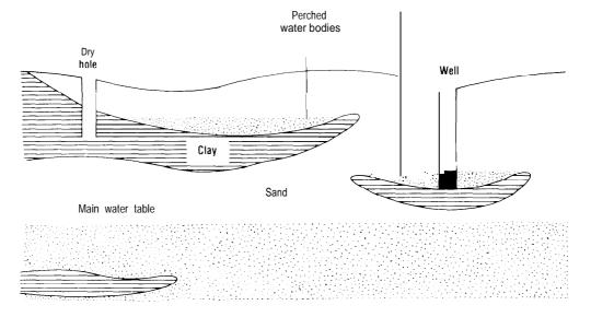
Figure 3-3-Perched Water Tables in Relation to the Main Water Table
