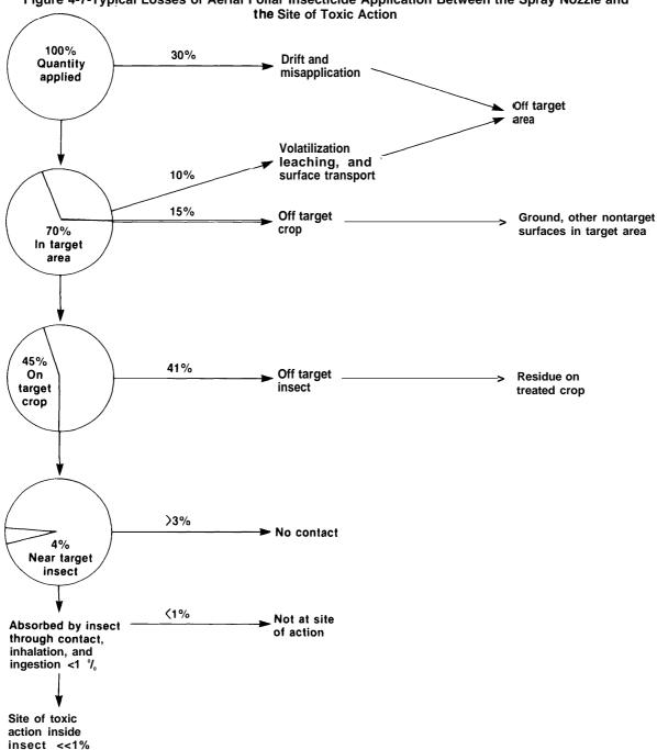
Figure 4-7-Typical Losses of Aerial Foliar Insecticide Application Between the Spray Nozzle and
